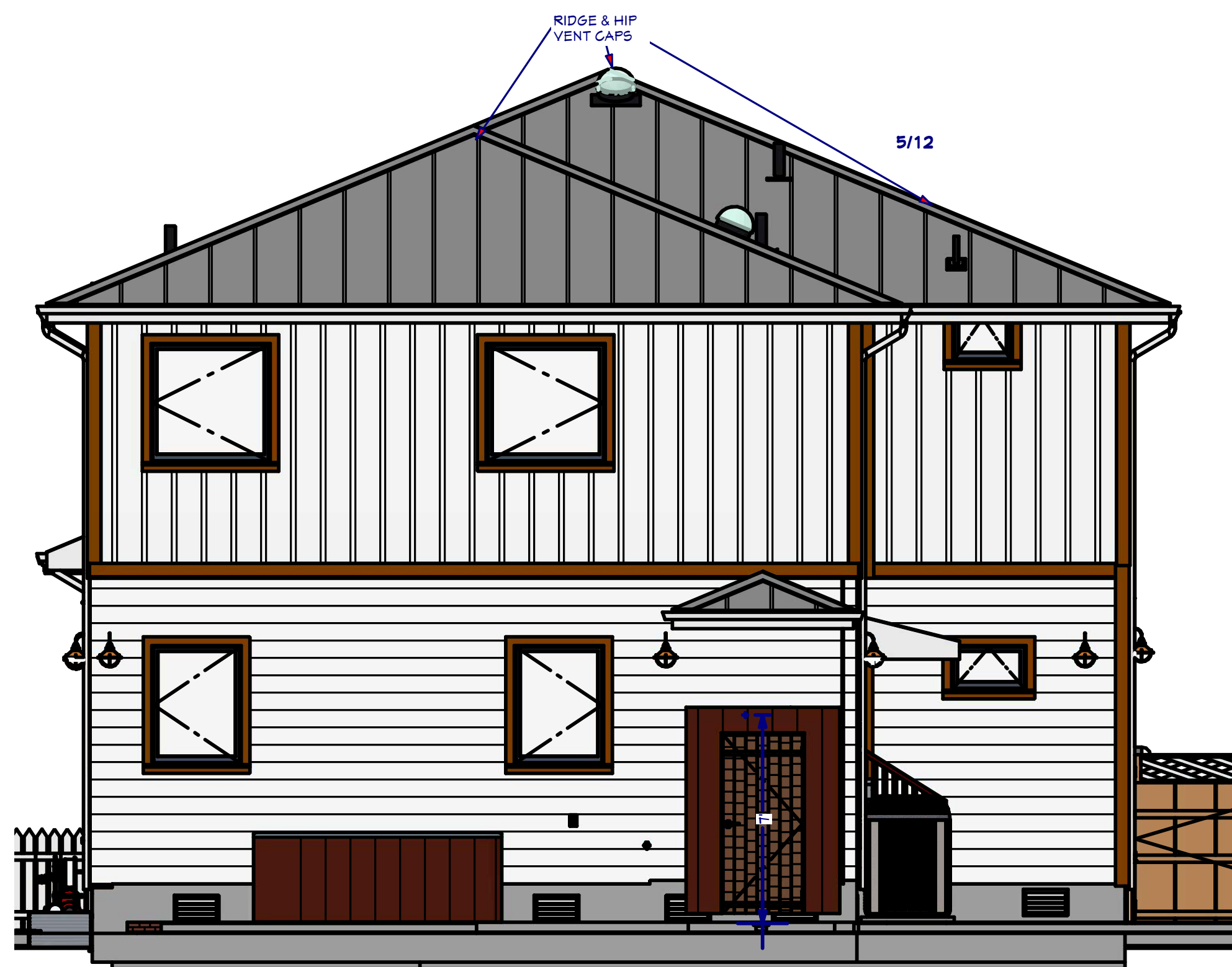
E-3 BACK ENTRY ( NORTH ) ELEVATION 1/4" = 1'
