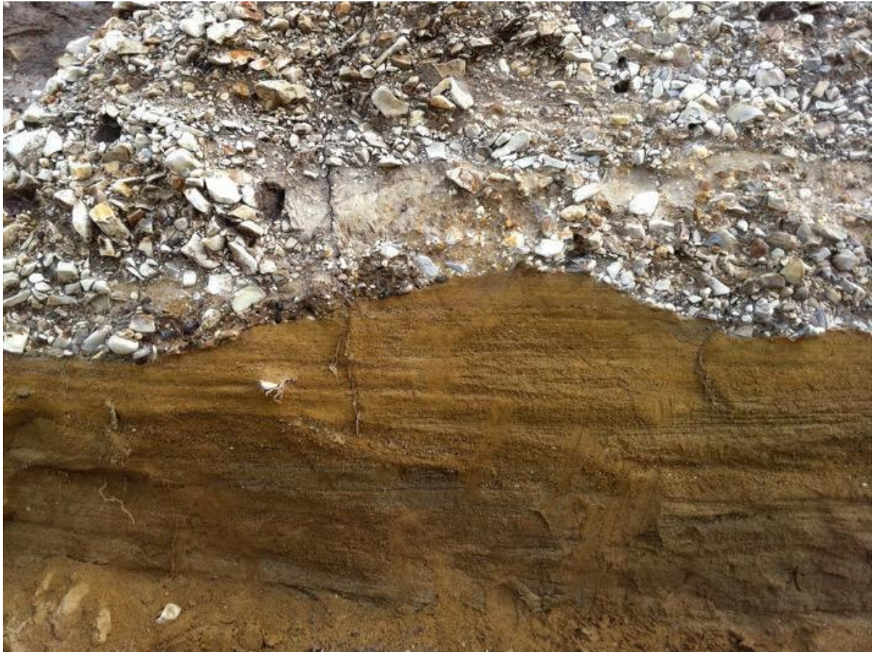
Figure 3-7. Section of bluff top terrace deposits at the end of Swift Street consisting of sand below and mudstone gravel and cobbles above
