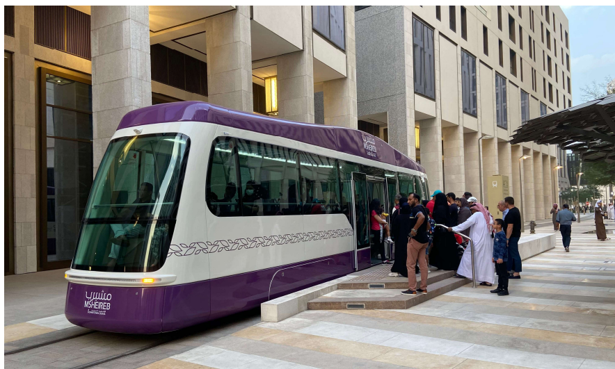
Figure 2.8: TIG/m MRV 3 - hydrogen fuel cell train operational in Doha, Qatar https://www.tig-m.com/products.html
